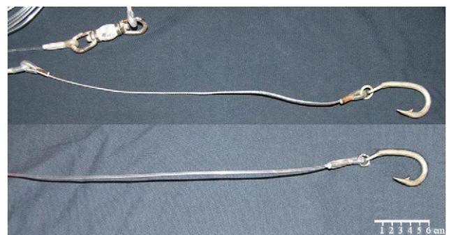
Fig. 2. The wire (above) and nylon (below) leaders used in the study. Also shown is a weighted swivel.
